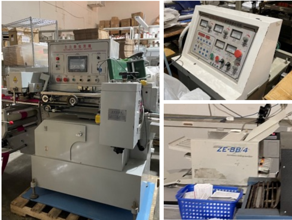
Figures 36-38 - Of the equipment in the Reedley Biolab, most was for packaging products. Pictured above, left and going clockwise: a PRC-origin automatic packing machine, a PRC-origin automatic separating and cutting machine, and an automatic folding machine. Source: City of Reedley.
